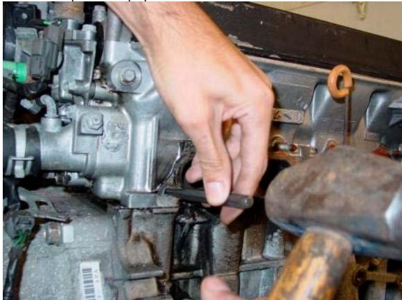
3. Drill a 1/8" hole in the stud. Take your time and do not push too hard. Be sure to use a liquid penetrant as lubricant so the drill bit will not overheat.
