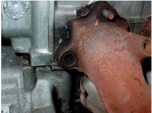
1. Remove the exhaust manifold and soak the broken stud with liquid penetrant.
