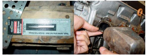
5. Unscrew the broken stud with a pair of vice grips attached to the extractor. Use lubricant if needed. Here's a pic of the broken stud removed.
